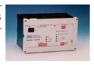
data to the transponder, decodes and checks the received transponder data and transmits it via a standard serial interface (RS232, RS422/485). The reader includes a Dynamic Auto Tuning (DAT) function that automatically tunes a standard antenna to resonance and keeps it tuned during operation.
